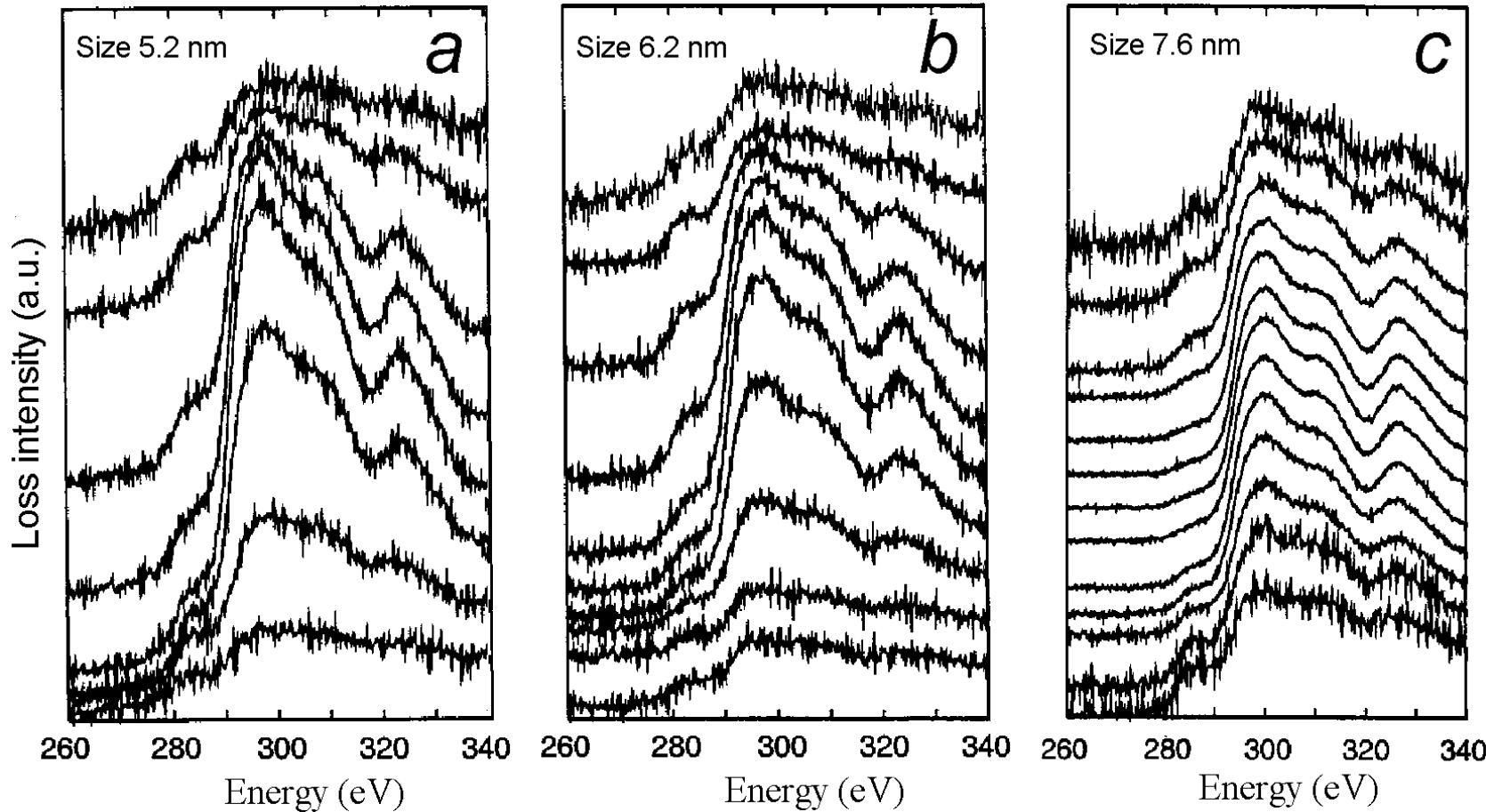
Line scan parallel electron energy loss spectrum for core-loss energy ranges for three DC particles of diameter (a) 5.2, (b) 6.2 and (c) 7.6 nm. Pre-peak (280–295 eV) characterises DC at the core-loss range
