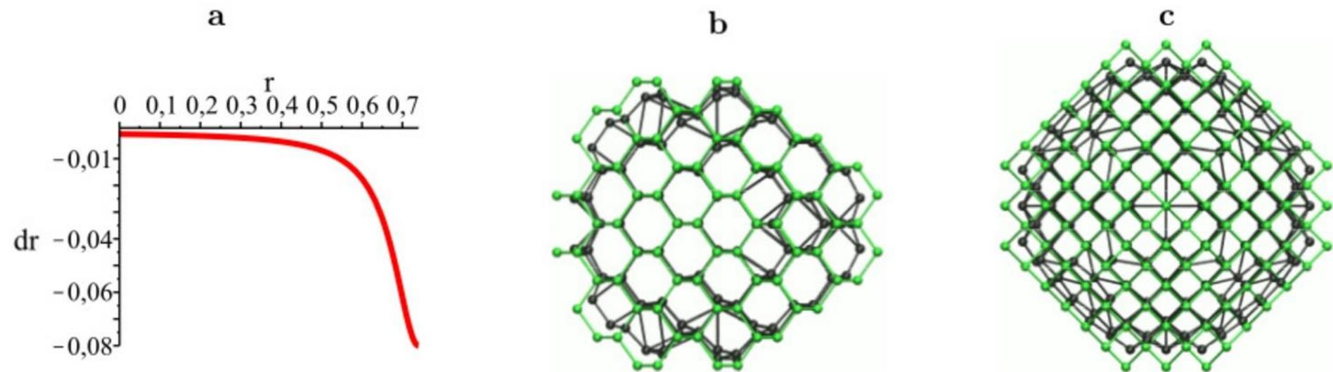
(a) Magnitude of the atom position shift to the origin vs. coordinate (fitted to the function (1) with parameters  $s = 10$ ,  $a = 0.08$ ). (b, c) Compression of the  $C_{302}$  diamond ball according to the function (1). Initial diamond ball (green) and deformed (black)
