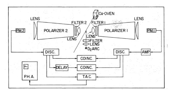
*Figure 4.* Schematic diagram of the apparatus and associated electronics used by Freedman and Clauser [11]. The distance between the detectors was 5 metres (m).
