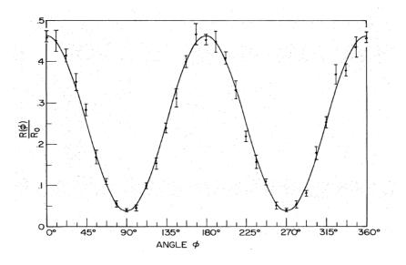
**Figure 5**. The experimentally measured ratio  $R(\phi)/R_0$  as a function of the angle  $\phi$  between the axes of the polarizers. The solid line is not a fit to the data points but the polarization correlation predicted by quantum mechanics. (From Freedman's PhD thesis, Experimental Test of Local Hidden-Variable Theories, Lawrence Berkeley National Laboratory, 1972.)
