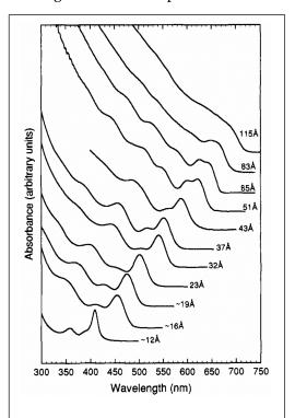
Fig. 4. Room-temperature optical absorption spectra of CdSe nanocrystallites dispersed in hexane and ranging in size from ~12 to 115 Å. Reproduced from C.B. Murray, D.J. Norris, and M.G. Bawendi, *J. Am. Chem. Soc.* **115**, 8706 (1993).
