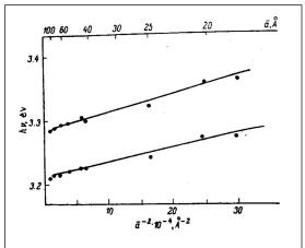
Fig. 2. Dependence of the spectral positions of exciton absorption lines at T = 4.2 K on the average radius  $\bar{a}$  of CuCl nanocrystals in glass. The energy of the absorption line increases proportional to  $\bar{a}^{-2}$ . Reproduced from A.I. Ekimov and A.A. Onushchenko, *JETP Lett* 1981, *34*, 345–349.
