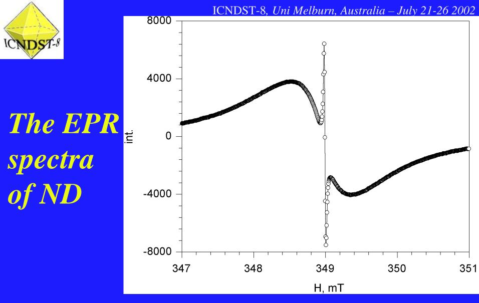
Central part of the EPR spectrum (EMX EPR Bruker) of ND in the NDC 10 nanocomposite with the Li standard (g = 2.0023). The scan and the modulation are 50 and 0.01 mT.
