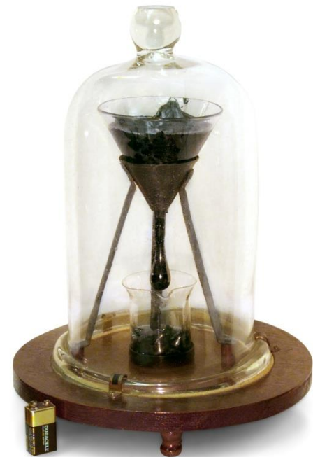
The University of Queensland pitch drop experiment
