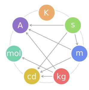
Current (2013) SI System: Dependence of base unitdefinitions on other base units (for example, the **metre**is defined in terms of the distance traveled by light in a specific fraction of a **second**)
