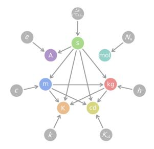
Proposed SI System: Dependence of base unit definitions on physical constants with fixed numerical values and on other base units that are derived from the same set of constants. Four further constants of nature should be defined to have exact values:
